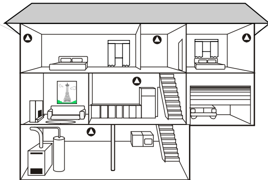
Figure 2: Recommended CO detector locations
